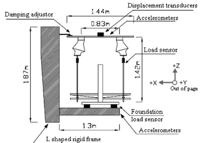
Fig. 4. Arrangements of the compliant model system.
