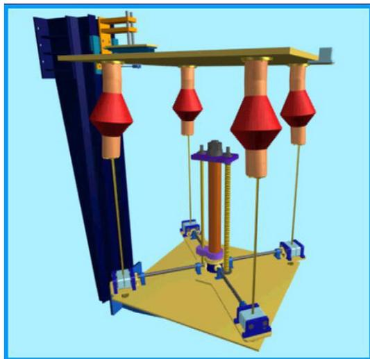
Fig. 2. 3D-plot of the compliant multi-legged model.
