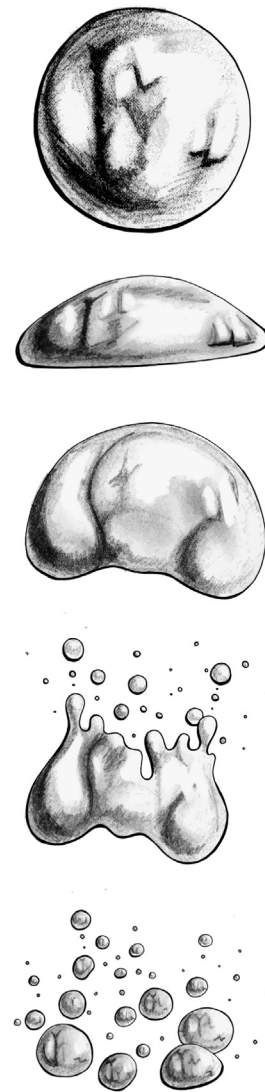
Fig. 2. A series of sketches by Kelsey Hemphill showing the breakup process of raindrops, based on photographs by Villermaux and Bossa (2009).
