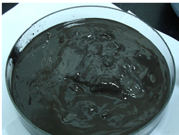
Fig. 1. Slurries from wire sawing of a Si wafer.
