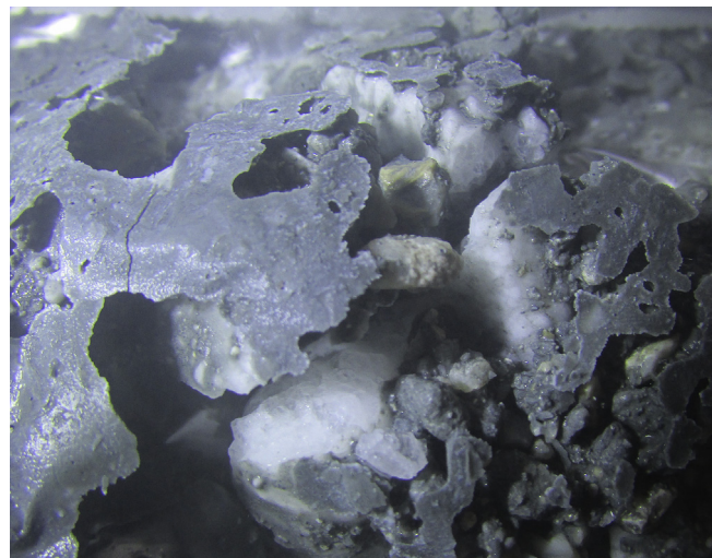
Figure 2. Gas hydrate Sample from PRM basin preserved in liquid nitrogen.
