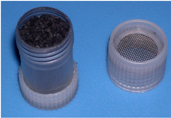
Fig. 1. Activated carbon filters.
