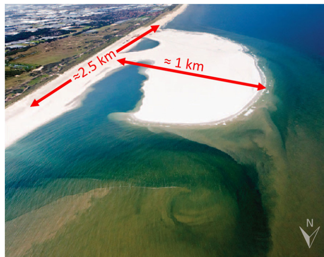
Fig. 1. Aerial photograph of the Sand Motor after completion (September 2011). Note the clouds of fine-grained material moving to the North. Picture courtesy of Rijkswaterstaat/Joop van Houdt.
