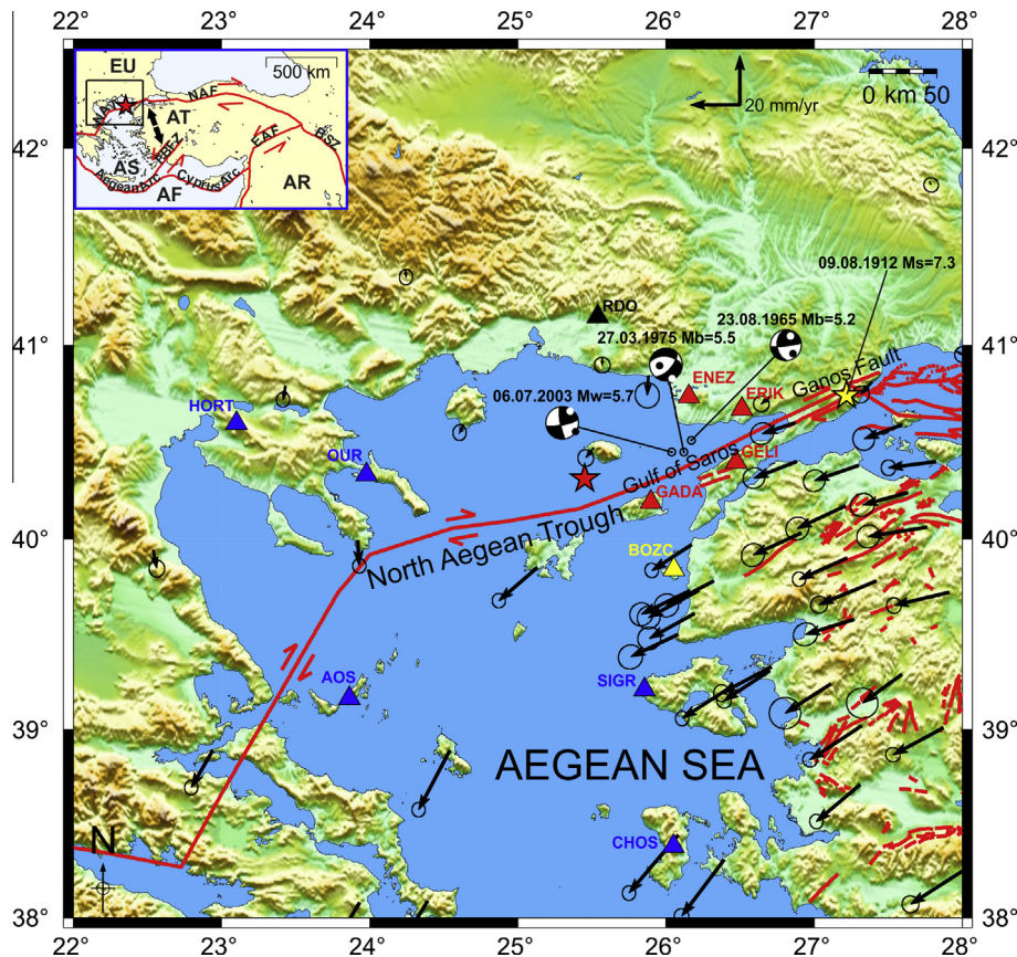
Fig. 1. Tectonic map of northern Aegean Sea showing GPS velocities with respect to Eurasia and 95% confidence ellipses for eastern Anatolia (McClusky et al., 2000; Reilinger et al., 2006). Seismically active faults are shown by red lines (Şaroğlu et al., 1992). Blue, red, black and yellow triangles with station codes depict locations of the AUTH, KOERI, NOA and AFAD broadband seismic stations, respectively. The epicenter of the 2014 NAS EQ is indicated by the red star. The yellow star indicates 9 August 1912 M_s = 7.3 Ganos EQ. For reference, focal mechanisms of the previous significant earthquakes are plotted (Karabulut et al., 2006; Tan et al., 2008). Black and white circles on beach-balls exhibit P and T -axes, respectively. The inset in the above left shows whole Turkey. Two closely spaced red single arrows display shear sense of major faults (NAT: North Aegean Trough, NAF: North Anatolian Fault, EAF: East Anatolian Fault, BSZ: Bitlis Suture Zone; FBFZ: Fethiye–Burdur Fault Zone). Boundaries (heavy colored red lines) of the Aegean Sea (AS) and Anatolian (AT) plates, which are surrounded by the African (AF), Arabian (AR) and Eurasian (EU) plates (Bird, 2003). The solid black rectangle shows the study area, which is enlarged in this figure. (For interpretation of the references to color in this figure legend, the reader is referred to the web version of this article.)
