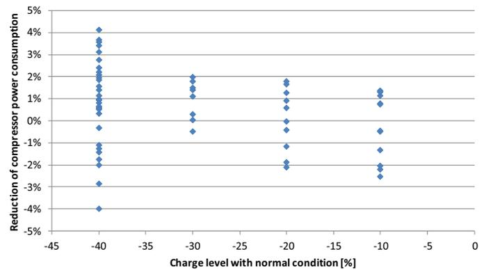
**Fig. 1.** Change of chiller power consumption with decreasing amount of refrigerant under a wide range of conditions (evaporator water outlet temperature from 277.35 K to 283.9 K, condenser water inlet temperature from 289.25 K to 303.36 K, evaporator water inlet temperature from 279.4 K to 289.5 K, evaporator water flow rate at  $49 \text{ m}^3 \text{ h}^{-1}$  and condenser water flow rate at  $61 \text{ m}^3 \text{ h}^{-1}$ ).
