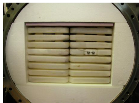
Fig. 3. Position of the instrumented PCM capsule in the tank as viewed from the outlet.
