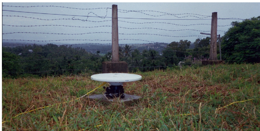
Fig. 1. PBLR monument and the antenna set up for 2003 and 2004 measurements. This stable setup is shown to showcase the minimized probability of setup errors. The monument consists of a steel bolt protruding out of a concrete pillar. In 2002 a Leica tribach was used with its adaptor. Vertical reference point is top of the concrete pillar. Antenna height in this occupation was 0.228 m. In 2003 a zephyr geodetic antenna was used along with a Trimble tribach. Antenna height in this occupation was 0.138 m. In 2004 a Leica choke ring was directly threaded to the bolt. The antenna height here was 0.0195 m.
