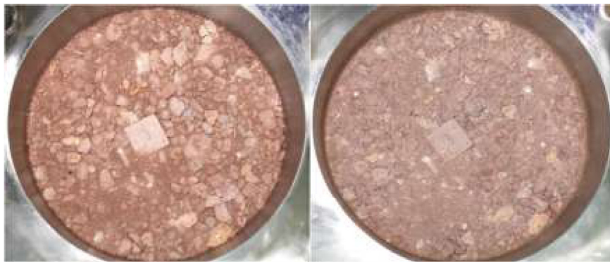
Fig. 1. (a) General scheme of the weathering test apparatus revised from Zhang et al. (2014); (b) Grain size distribution for materials used in tests (Zhang et al., 2015); (c) A specimen before and after weathering.
