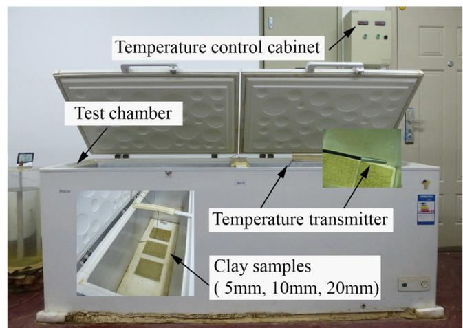
**Fig. 1.** Image of experimental set-up for the freezing–thawing tests.
