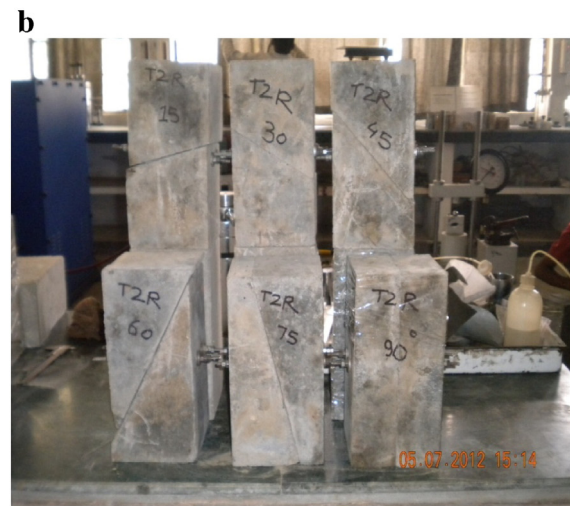
Fig. 2. a. Joint and bolt configuration in concrete specimens. b. Prepared reinforced specimens of concrete.
