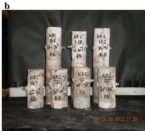
Fig. 1. a. Configuration of specimens of natural rock. b. Prepared reinforced specimens of natural rock.
