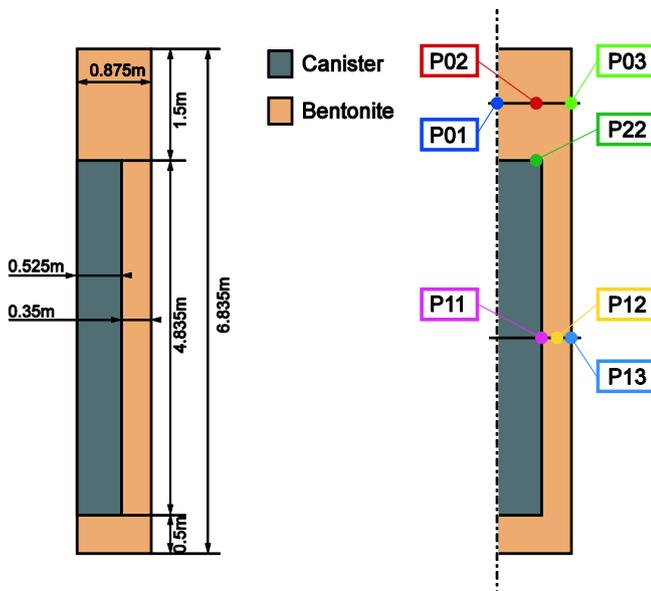
Fig. 1. Geometry of the considered deposition hole, location of monitoring points.
