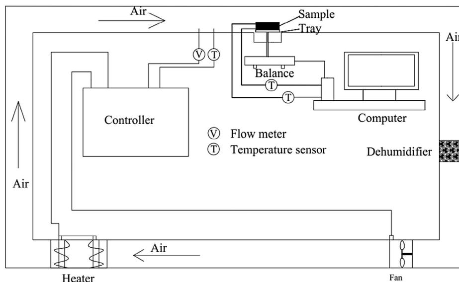
Fig. 1. Convective dryer setup.
