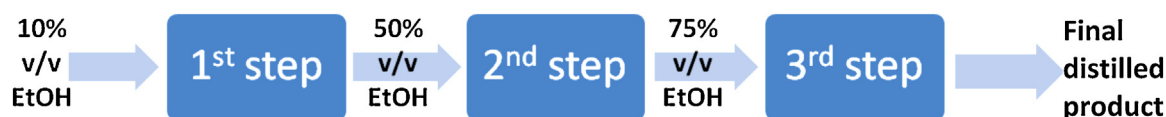
Fig. 1 – Steps in distillation process for both OAHD and HD: second and third steps were performed in current study, first step is described by Gavahian et al. (2016a).
