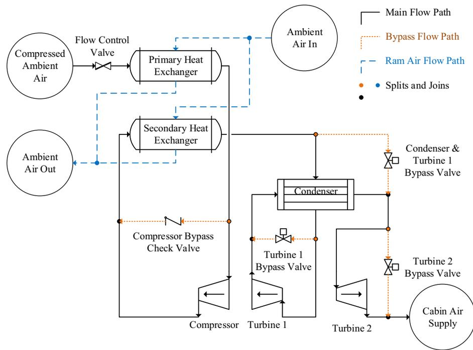
Fig. 1. Typical aircraft ECS piping and instrumentation diagram [3].
