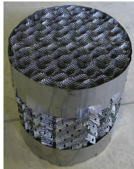
Fig. 2. Traditional perforated corrugated packing.
