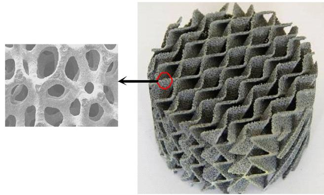
Fig. 1. SiC ceramic foam corrugated packing.
