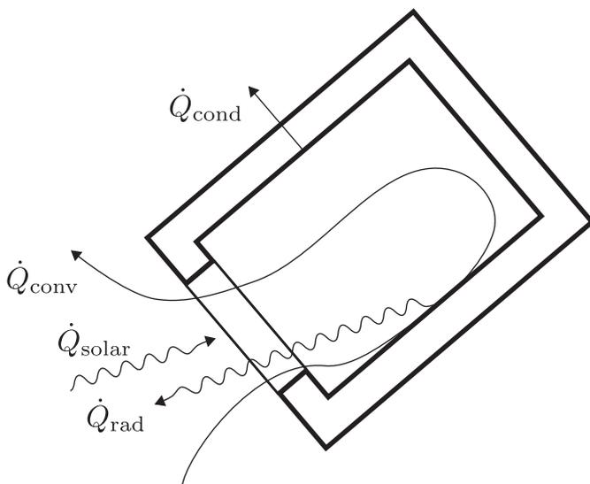
Fig. 1. The diagram shows the different heat loss mechanisms which reduce the usable share of the absorbed solar radiation  $\dot{Q}_{solar}$ .
