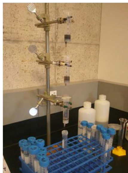
Fig. 1. Schematics of the chromatographic separation process (top), and actual modified apparatus (bottom). (colour on line)
