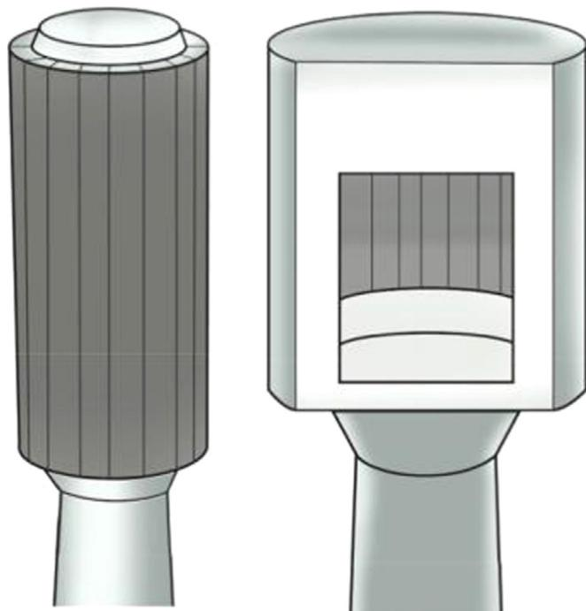
Fig. 1. Schematics of tubular (left) external and cavity receivers (right).
