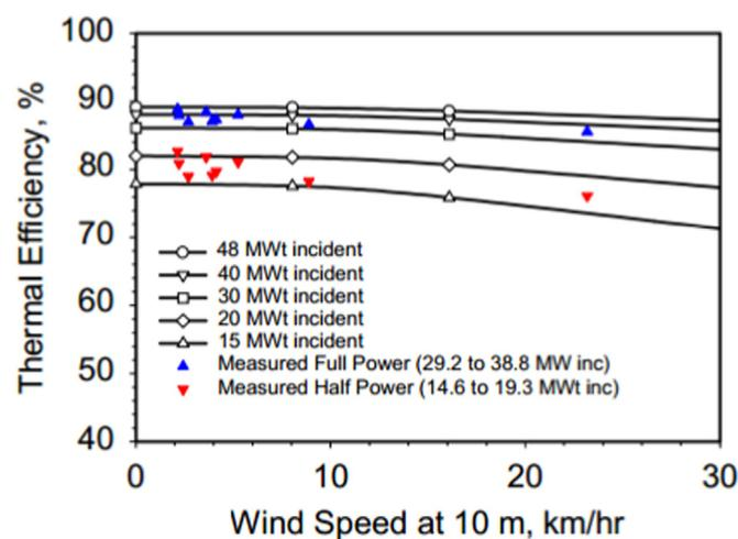
Fig. 2. Modeled and measured receiver efficiency as a function of wind speed for Solar Two [5].
