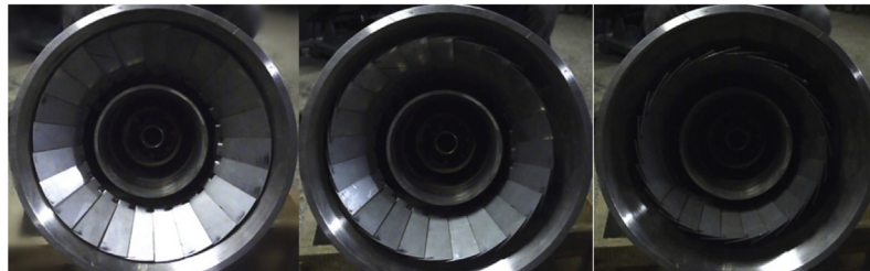
(a) Burner spouts of three different ISA flaring angles
