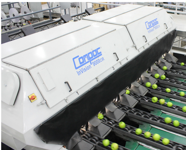
Fig. 1. An inspection zone enclosed by a cabinet which makes the calibration volume of interest inaccessible. The produce are moved and rotated by the conveyor under the inspection system.
