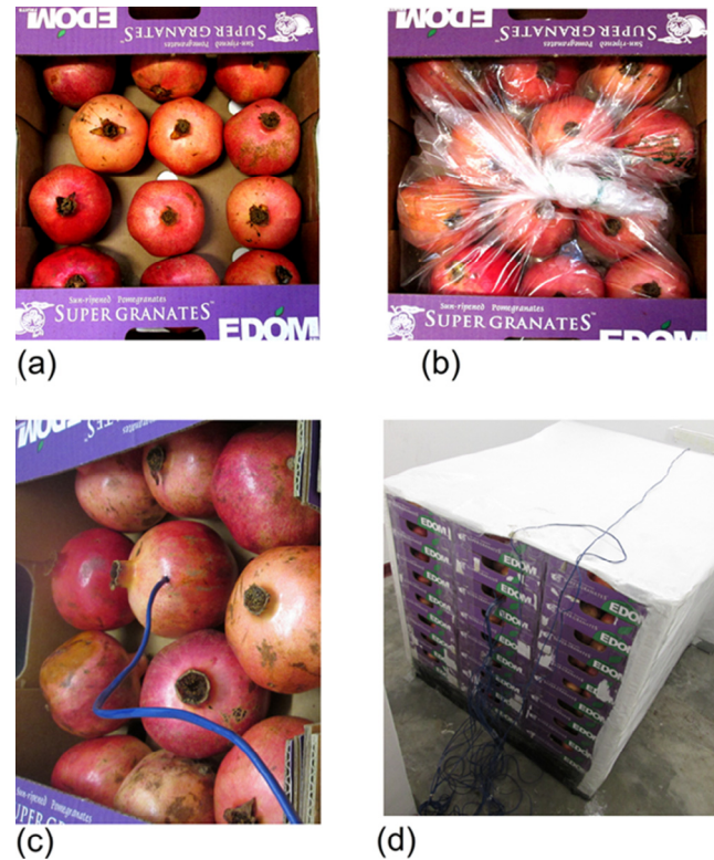
Fig. 1. Components of the experimental setup. Pomegranates in the CT2 packaging box, with no lining (a), with liner (b), thermocouple inserted to fruit centre to measure pulp temperature (c) and stack ready for the FAC test (d).
