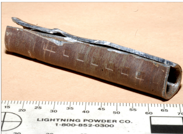
Fig. 3. A lead sheet with impression marks, after being taken off the sample rod.
