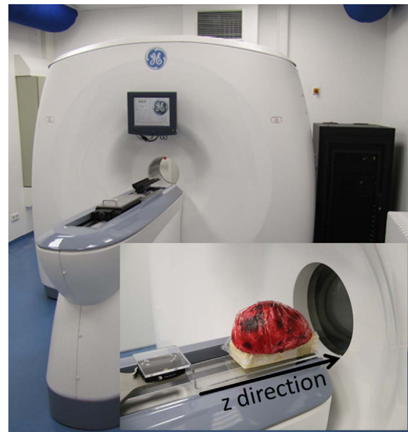
Fig. 1. Photograph of the eXplore Locus Ultra CT scanner. The inset image shows an excised calvarium positioned on a sponge on the scanner’s specimen holder.
