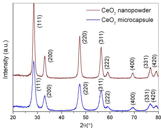
Fig. 1. XRD patterns of  $\text{CeO}_2$  nanopowder and N-doped  $\text{CeO}_2$  microcapsule.
