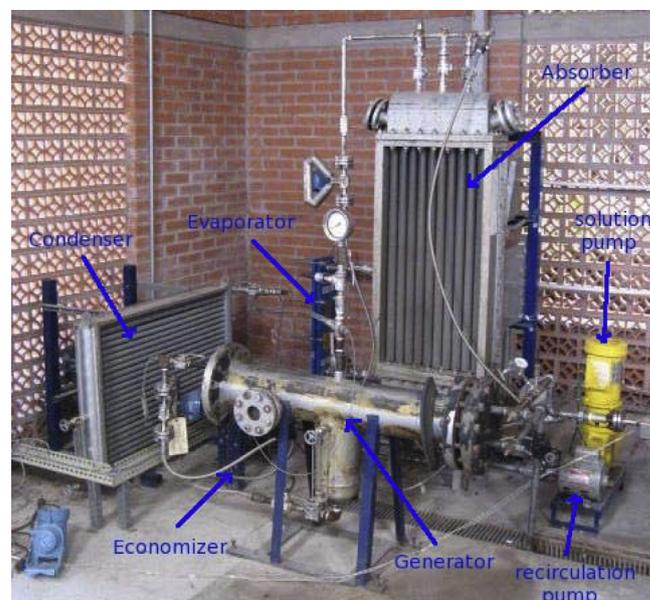
Fig. 1. Absorption cooling system.
