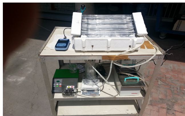
Fig. 1. Solar photoreactor adopted.
