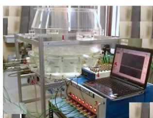
Scaled-down cold flow model of BOF vessel
