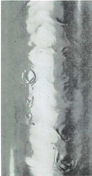
Fig. 1. Experimental picture in annular two-phase flow (Cousins and Hewitt, 1968) of depositing liquid film for a mean gas velocity of 28 m/s.
