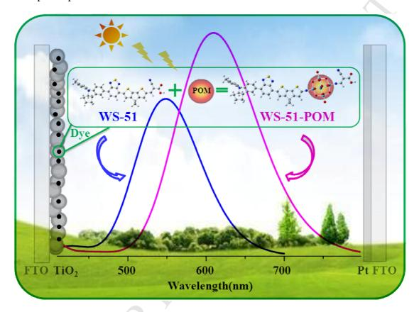
Four D-A- $\pi$ -A hybrids were designed by introducing polyoxometalate for improving photovoltaic performance.
