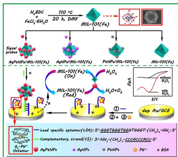
**Scheme 1.** Schematic illustration of the fabrication process of the proposed  $Pb^{2+}$  electrochemical aptasensor, together with the preparation of different signal probes, and the mechanism of the signal amplification in the electrode interface.
