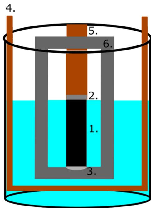
Fig. 1. Schematic drawing of the experimental setup consisting of (1) CNT film, (2) silver paste electrical contact, (3) glue, (4) Copper sheet, (5) Copper conductor sheet, and (6) PVC sample holder.
