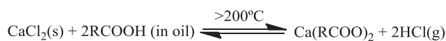
Fig. 1. HCl formation through the hydrolysis of native metal chlorides or through the reaction with naphthenic acids [3]
