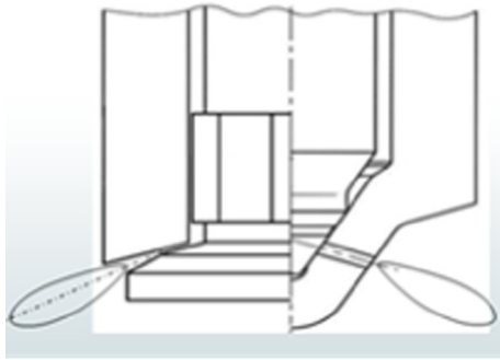
Fig. 2. Schematic view of geometrical features of HCN (left) compared with a conventional MHN (right).
