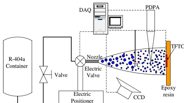
Fig. 1. Schematic of the experimental system.
