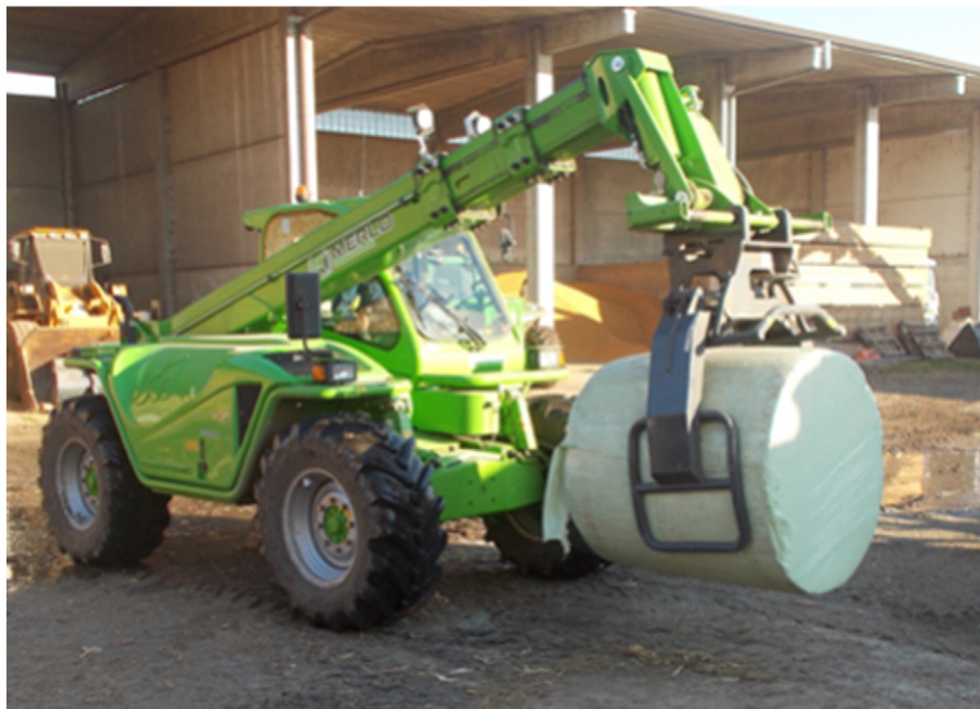
Fig. 2. Telescopic handler used to move the wrapped bales.
