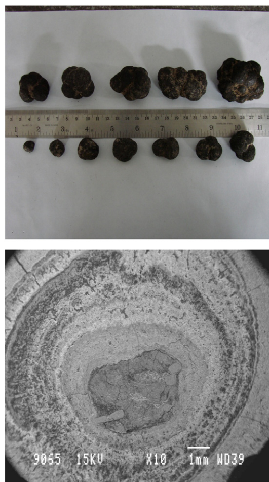
Fig. 1. (a) Manganese nodules obtained from Central Indian Ocean Basin and (b) magnified view of cross-section of manganese nodule.
