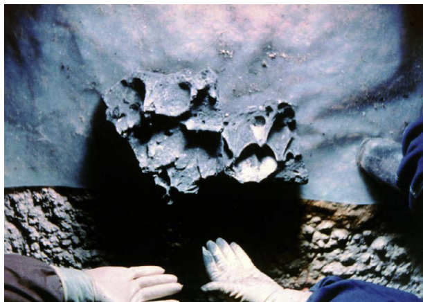
Fig. 1. Large fragment of Chernobyl “lava” prepared for packing and delivery to Leningrad. Photo had been taken by B. Burakov inside “Shelter” in 1990.
