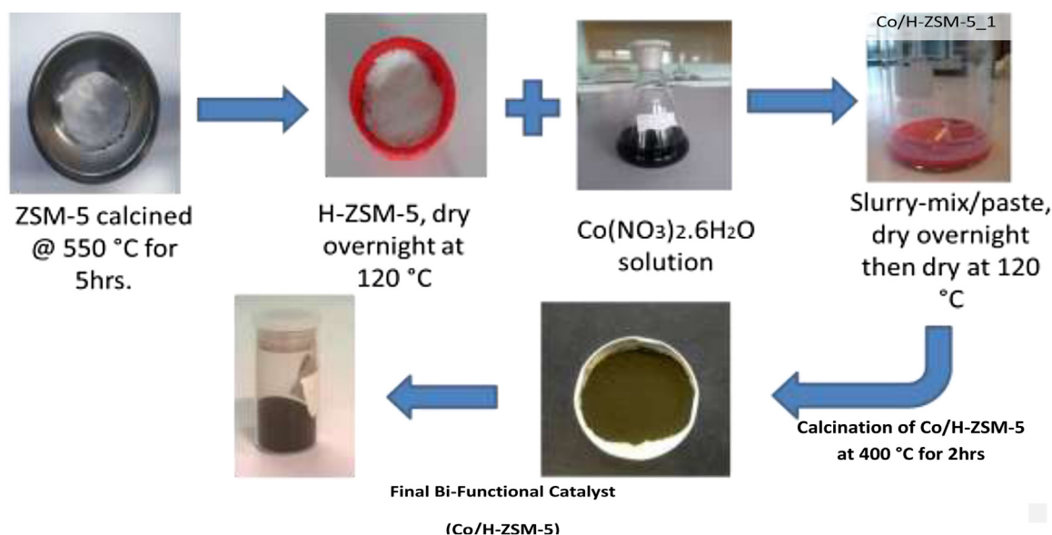
Fig. 1. Scheme for the synthesis of the Co/H-ZSM-5 catalyst. The same procedure was followed for the preparation of the Co/SiO 2 catalyst, except the step that involves the conversion of ammonium form-ZSM-5 to H-ZSM-5.
