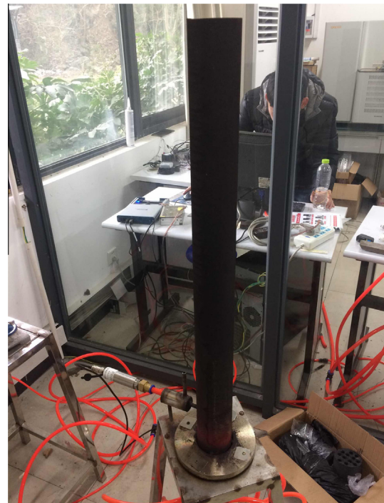
Fig. 1. Photo of a closed-open standing-wave thermoacoustic combustor with a total length of L = 800 mm.
