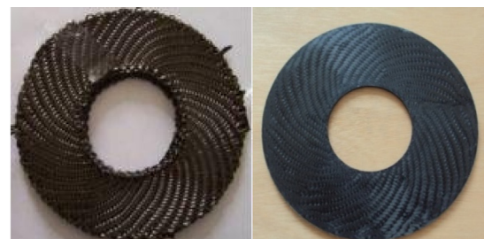
(b) Spiral twill woven fabric and stacked composites disk
