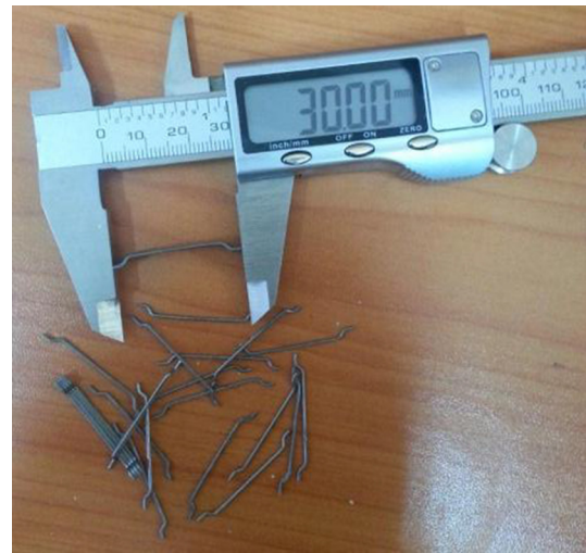
Fig. 2. Steel fibers with hooked-ends.
