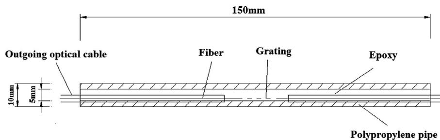
**Fig. 1.** Size of pipe for FBG sensors.
