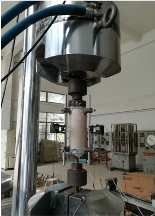
Fig. 1. Instrumented concrete cylinder.
