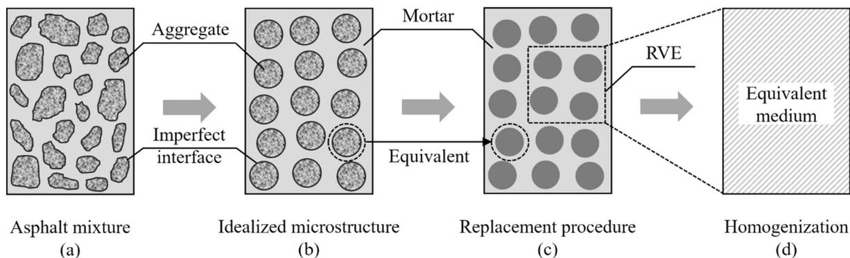
Fig. 1. Schematic representation of microstructure idealization process.
