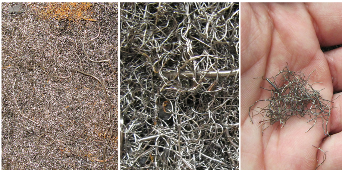
Fig. 1. Recycled steel fibers derived from waste tires.
