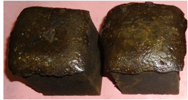
Fig. 1. SiMn slag based alkali activated hardened sample.
