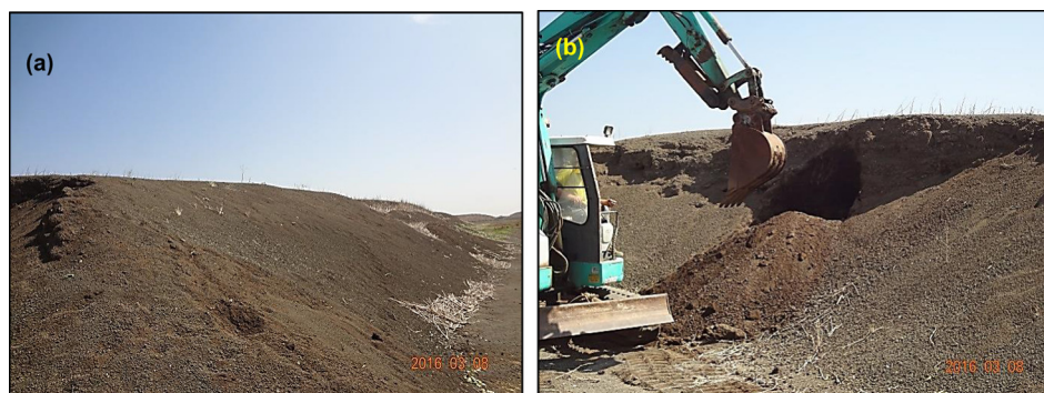
Fig. 1. (a) WTP Stockpile No 10; (b) collecting about 1 m 3 of biosolids from WTP stockpile No 10.
